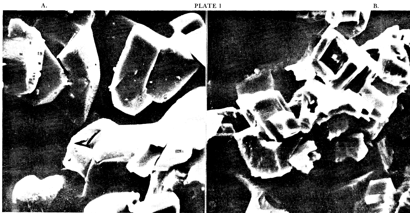
Scanning electron photomicrographs of reagent grade calcite partially dissolved in seawater ( \times 5000 ). (After Berner and Morse, 1974.) (A) Diffusion-controlled dissolution at \text{pH} = 3.9 , P_{\text{CO}_2} = 10^{-2.5} (80 percent of original mass removed by dissolution). (B) Surface reaction-controlled dissolution at \text{pH} = 6.0 , P_{\text{CO}_2} = 10^{-2.5} (60 percent of original mass removed by dissolution).
